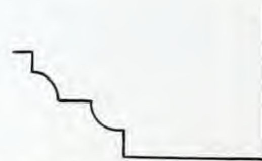
No. 929.—Angle moulding ; any size to suit.
